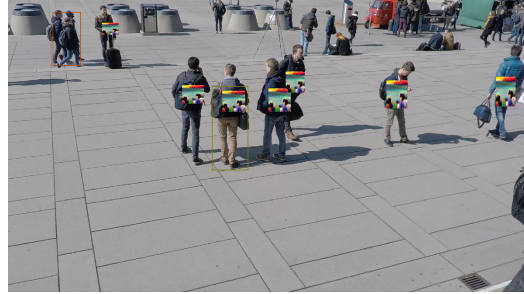
Figure 2. Sample of the Wildtrack view 7 detection results with the patch applied after geometric transformation
