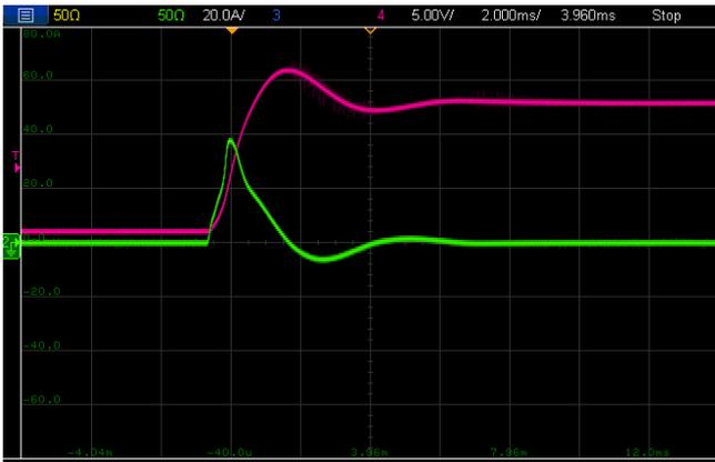
Fig. 9: Initial inrush current without start-up procedure.
