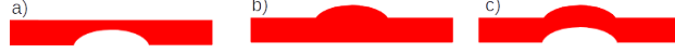
Figure 7: Different kinds of pixels detected as irregular: a) concave only irregularity, b) convex only irregularity, c) symmetric irregularity.
