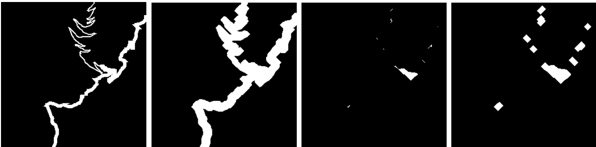
Figure 8: Steps for detecting coalescent pixels, from left to right: initial image, dilation, erosion, dilation.
