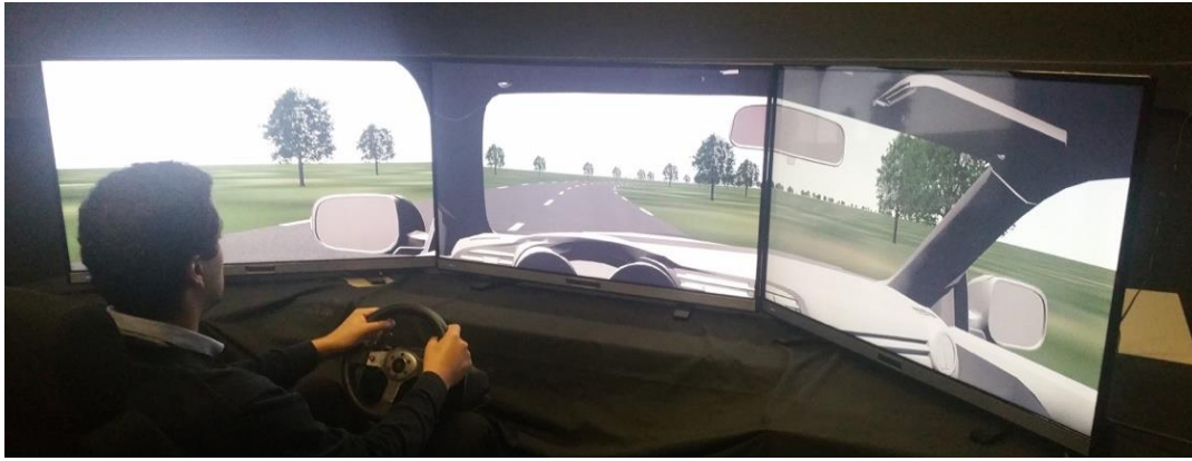
Figure 1. Illustration of the low-cost driving simulator with a virtual full-scale cab displayed in the visual scene.
