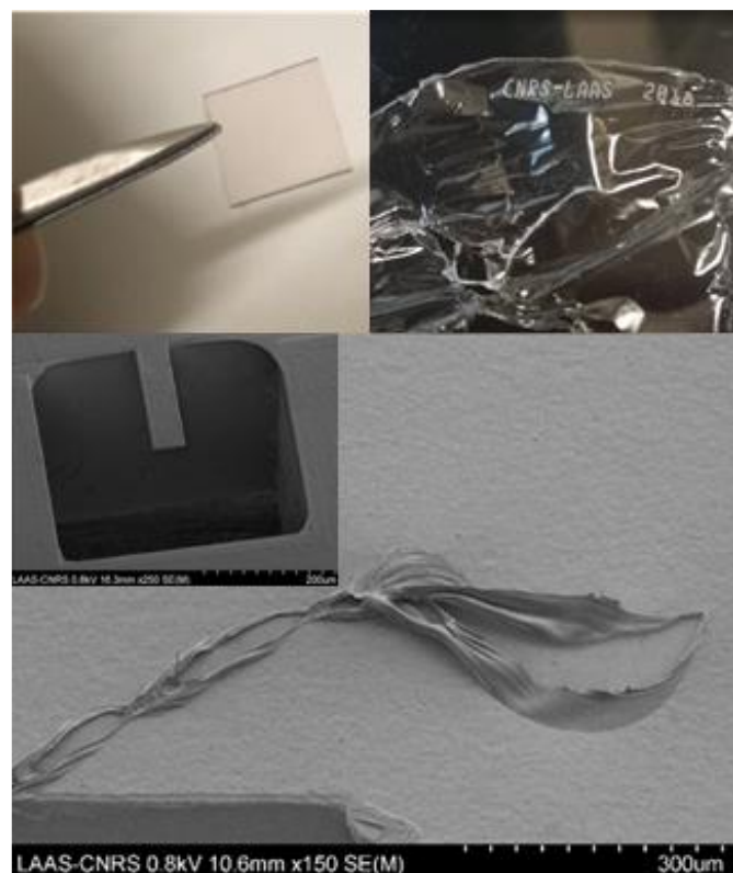
Figure 1. Top panel: Representative photographs of a P(VDF-TrFE) coated glass substrate and a 10 \mu\text{m} thick freestanding film. Bottom panel: SEM images of a 800 nm thick P(VDF-TrFE) coating deposited on a microstructure. (A scratch was made to reveal the coating.)
