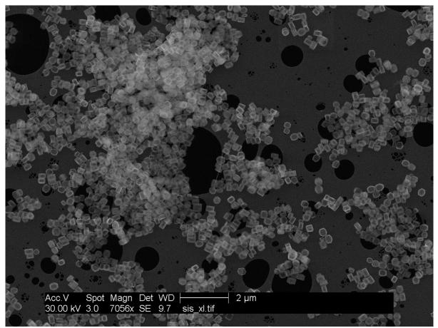
Figure S5. Large SEM image of small single hollow crystals
