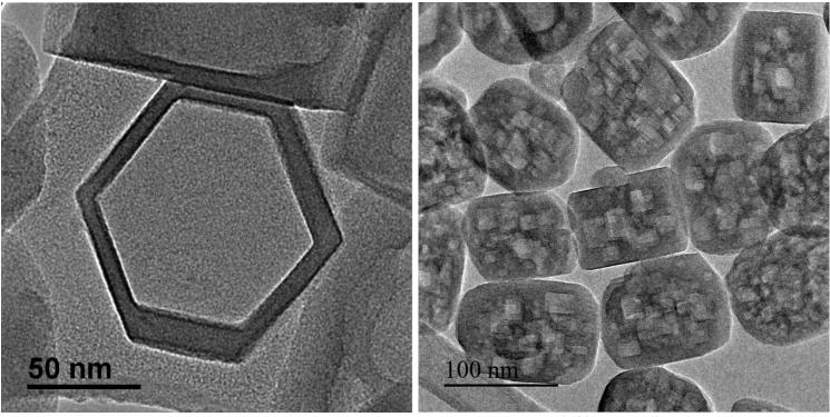
Figure S2. TEM images demonstrating crystalline pattern in small single (left) and multi (right) hollow crystals
