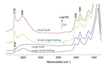
Figure S6. DRIFTS spectra collected over the various samples at 150 °C after drying at 250 °C for 30 min
