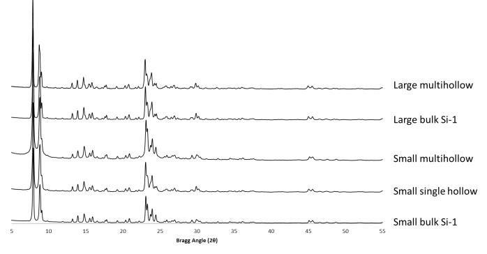
Figure S1. XRD pattern of silicalite-1 samples
