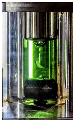
Figure 4: Picture of the cell with the \text{CO}_2 + \text{N}_2\text{O}_4 mixture at low temperature
