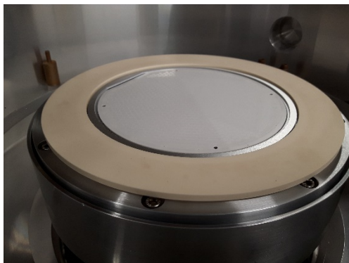
Figures: Wide range electrostatically clamped wafer table (left) Thermal simulation (right)
