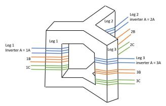
Fig. 3: Inverters phases and windings arrangement on the transformer
