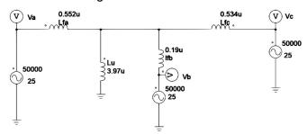
Fig. 12: Psim circuit used for the simulation of the T-model
