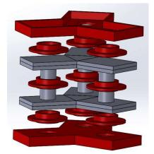
**Fig. 2:** Exploded view of the magnetic component (grey) and its plastic supports (red)
