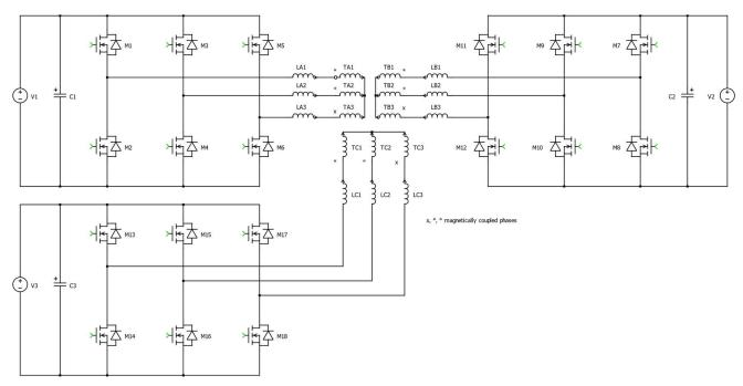
Fig. 1: Complete schematic of the converter
