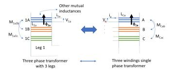
**Fig. 5:** Three phase to single phase transformer conversion
