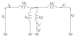
Fig. 7: T-model of the three windings transformer
