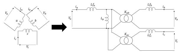
Fig. 6: Full model of the three windings transformer
