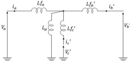
Fig. 7: T-model of the three windings transformer
