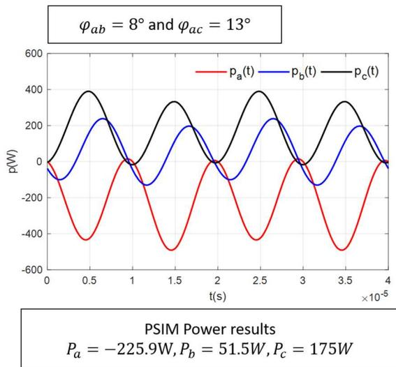
**Fig. 13:** Simulation for identical phase shifts between  $V_a$  and  $V_b$  and  $V_c$ .
