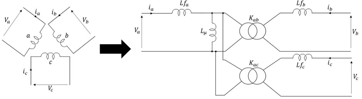
**Fig. 6:** Full model of the three windings transformer
