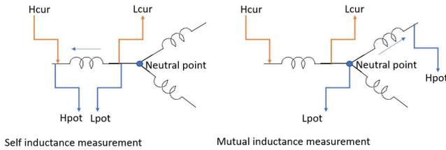
Fig. 10: Measurement schematics
