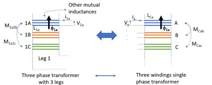
**Fig. 5:** Three phase to single phase transformer conversion
