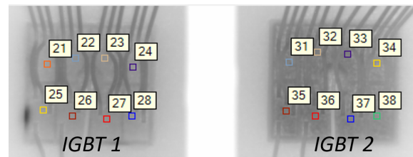
Fig. 4: Infrared thermography measurement
