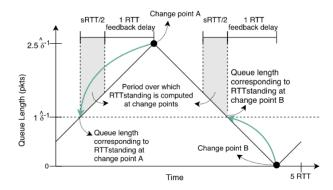
Fig. 2: COPA mechanism described in [6]. The aim is to stabilise the queue length around  $\delta^{-1}$ .
