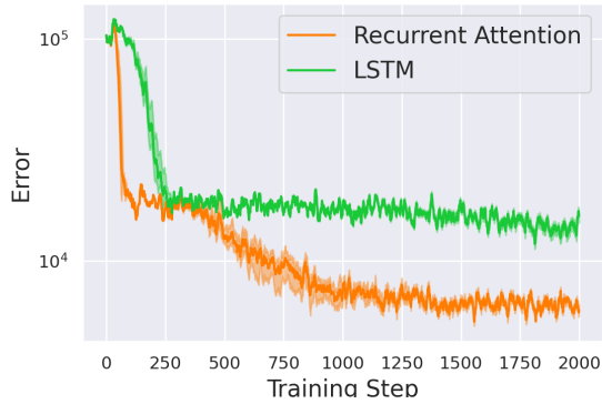
(a) Training loss. The colored envelopes represents the maximal and minimal errors for 10 trained models.
