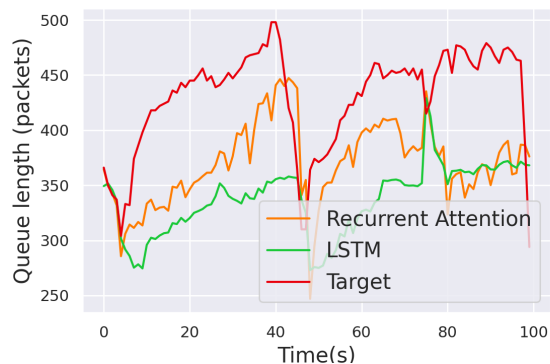
(b) Estimation of of the bottleneck load (with emulation) using LSTM and Attention architectures.
