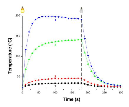
Figure 5. Temperature versus time of TMPTA-based polymers. Irradiations are performed at 1064 nm (2.5 W.cm<sup>-2</sup>) from t = 0 s to t = 180 s and stopped from t = 180 s. (1) TMPTA-based polymer without heater. (2) TMPTA-based polymer in presence of IR-813 (0.1%<sub>wt</sub>). (3) TMPTA-based polymer in presence of IR-940 (0.1%<sub>wt</sub>). (4) TMPTA-based polymer in presence of IR-1064 (0.1%<sub>wt</sub>).
