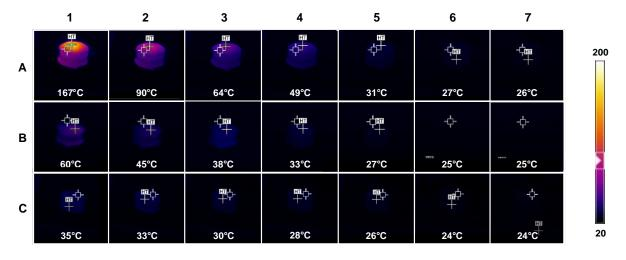
Figure 2. Thermal imaging camera pictures after NIR irradiation. Pictures are taken (1) 0 s; (2) 10 s;
