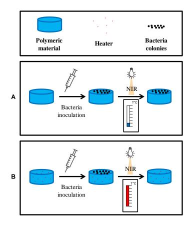
Scheme 2. Bacteria annihilation using NIR irradiation. (A) Polymer sample without heater. (B) Polymer sample with heater.
