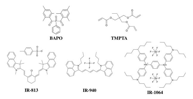
Scheme 1. Chemical structures of the monomer (TMPTA), photoinitiator (BAPO) and NIR heaters (IR-813, IR-940 and IR-1064) used in this study.
