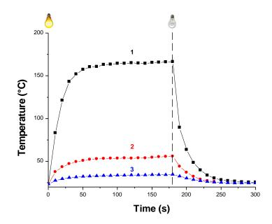
**Figure 3.** Temperature versus time of TMPTA-based polymers. Irradiations are performed at 785 nm from t = 0 s to t = 180 s and stopped from t = 180 s. (1) TMPTA-based polymer in presence of IR-813 (0.1%<sub>wt</sub>) at 2.55 W.cm<sup>-2</sup>. (2) TMPTA-based polymer in presence of IR-813 (0.1%<sub>wt</sub>) at 0.4 W.cm<sup>-2</sup>. (3) TMPTA-based polymer without heater at 2.55 W.cm<sup>-2</sup>.
