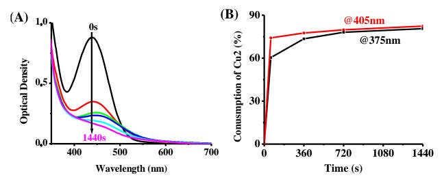
**Figure 11.** (A) Photolysis of Cu2 with Iod  $(10^{-2} \text{ M})$  upon irradiation @375 nm. (B) Consumption of Cu2 with irradiation @375 nm and 405 nm.
