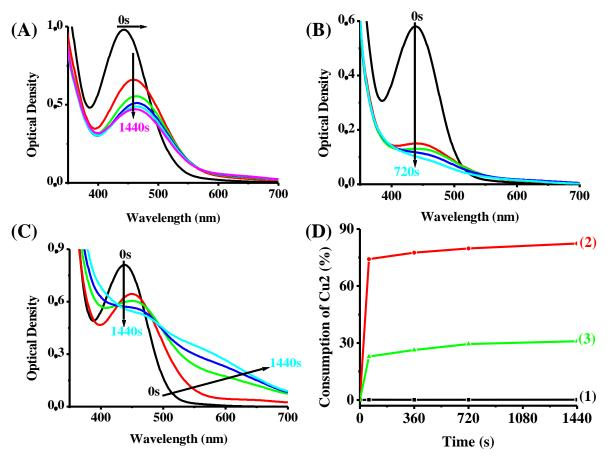
**Figure 10.** Photolysis experiments of (**A**) Cu1 with Iod salt  $(10^{-2} \text{ M})$ , (**B**) Cu2 with Iod salt  $(10^{-2} \text{ M})$  and (**C**) Cu2/Iod/NPG  $(10^{-2} \text{ M})$  upon exposure to LED at 405 nm. (**D**) Consumption percentage of Cu2: (1) alone, (2) with Iod, (3) with Iod/NPG.
