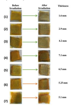
**Figure 8.** Free radical photopolymerization for the photocomposite synthesis upon near-UV irradiation at 395 nm (4 W·cm $^{-2}$ ) using Cu2/Iod/NPG (0.1%/1%/1% w/w/w) in TA [(1)–(4)], (5)) Cu2/Iod/NPG (0.1%/1%/1% w/w/w) in TMPTA, (6) Cu1/Iod/NPG (0.1%/1%/1% w/w/w) in TMPTA and (7) Cu1/Iod/NPG (0.1%/1%/1% w/w/w) in TA.
