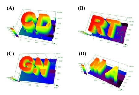
**Figure 9.** 3D patterns produced by free radical photopolymerization of acrylate functions (TA or TMPTA) using a laser diode at 405 nm and their characterization by numerical optical microscopy: (**A**) Cu2/Iod/TMA (0.057%/1%/0.46% w/w/w) in TA, (**B**) Cu1/Iod/TMA (0.058%/0.506%/0.44% w/w/w) in TMPTA; (**C**) Cu2/Iod/TMA (0.048%/0.65%/0.259% w/w/w) in TA and (**D**) Cu1/Iod/TMA (0.05%/0.5%/0.305% w/w/w).
