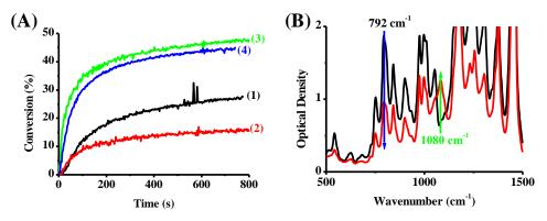
**Figure 6.** (**A**) Cationic polymerization (CP) profiles of epoxy functions (thin sample) vs. irradiation time upon exposure to LED at 405 nm: (1) Cu1/Iod  $(0.1\%/1\% \ w/w)$ , (2) Cu2/Iod  $(0.1\%/1\% \ w/w)$ , (3) Cu1/Iod/NVK  $(0.1\%/2\%/3\% \ w/w/w)$  and (4) Cu2/Iod/NVK  $(0.1\%/2\%/3\% \ w/w/w)$ . (**B**) IR spectra recorded before and after polymerization. Irradiation starts at t = 10 s.
