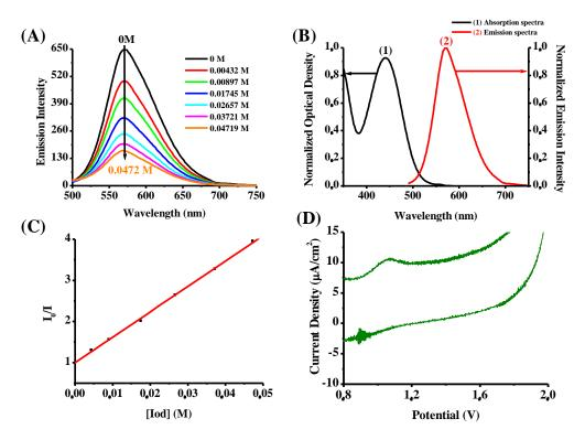
**Figure 12.** (**A**) Fluorescence quenching of Cu2 by Iod salt, (**B**)  $E_{S1}$  determination for Cu2, (**C**) Stern–Volmer coefficient determination of Cu2 quenched by Iod and (**D**) oxidation potential determination of Cu2.
