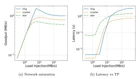
Fig. 5: Network saturation while injecting 3MB, Round Robin w/ variable frequency.
