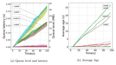
Fig. 6: Stress load injection of 0.5MB, Round Robin ( $\lambda = 10$ ).
