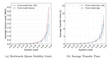
Fig. 3: Model validation for average steady state queue level and transfer time for arbitrary particle during system load saturation.
