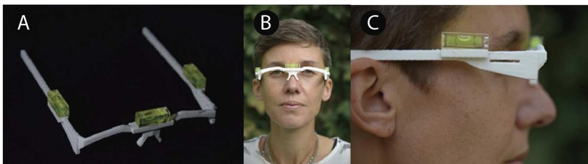
**Figure 2:** The prototype ensuring the horizontality of the reference plane on both axes. A: the mount with bubble levels; B: an example of use; C: the slot on the side of the frame allows the eyes to be aligned.
