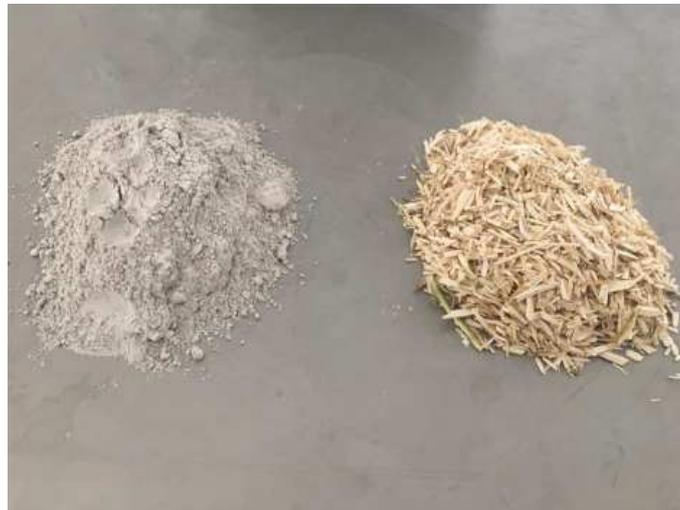
Figure 2. *Lime and hemp used in the process*
