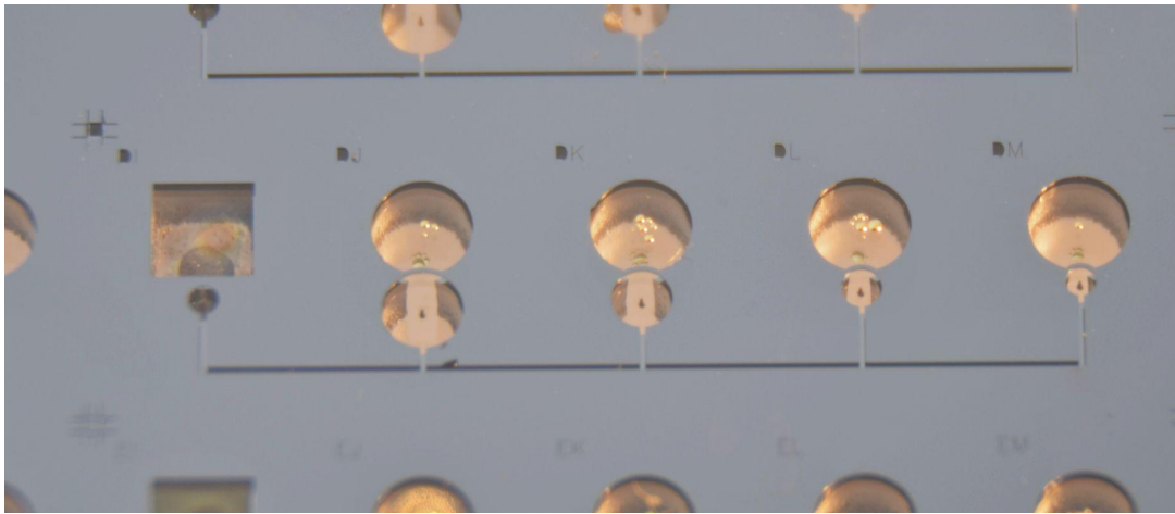
Figure 1: An array of microfabricated cells featuring make-seals connected to a common source of cesium (before sealing and dicing).
