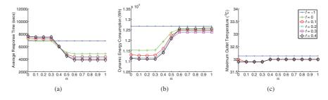
Fig. 8. Multi-objective scheduling for  $H_{i,j}^{T,RE} = \langle \overline{H}_{i,j}^T(f), \alpha \overline{H}_{i,j}^R + (1-\alpha) \overline{H}_{i,j}^E \rangle$  with different f and  $\alpha$  at 20% load intensity.
