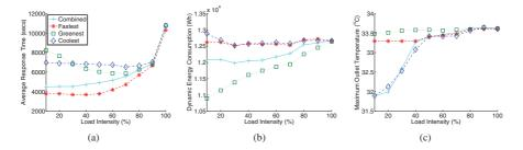
Fig. 9. Multi-objective scheduling for  $H_{i,j}^{T,RE} = \langle \overline{H}_{i,j}^{T}(f), \alpha \overline{H}_{i,j}^{R} + (1-\alpha) \overline{H}_{i,j}^{E} \rangle$  with f = 0.4 and  $\alpha = 0.5$  at different load intensities.
