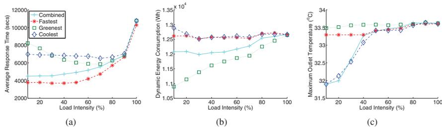
Fig. 9. Multi-objective scheduling for  $H_{i,j}^{T,RE} = \langle \overline{H}_{i,j}^T(f), \alpha \overline{H}_{i,j}^R + (1 - \alpha) \overline{H}_{i,j}^E \rangle$  with  $f = 0.4$  and  $\alpha = 0.5$  at different load intensities.
