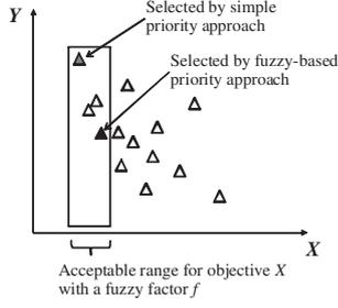
Fig. 1. The fuzzy-based priority approach in dual-objective scheduling.
