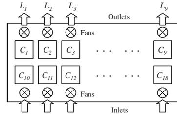
Fig. 2. The layout of the RECS server system.
