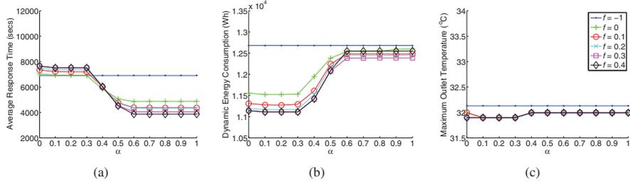
Fig. 8. Multi-objective scheduling for  $H_{i,j}^{T,RE} = (\bar{H}_{i,j}^T(f), \alpha \bar{H}_{i,j}^R + (1 - \alpha) \bar{H}_{i,j}^E)$  with different  $f$  and  $\alpha$  at 20% load intensity.
