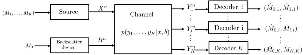
Fig. 2. Source-backscatter device to K-receivers discrete channel model
