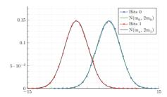
Fig. 1: Probability density function of the LLRs at the output of GSM GMSK decoder vs symetric Gaussian distribution when a priori mutual information is 0.5.  $m_O$  (resp.  $m_1$ ) is the expected value of LLRs associated with bits 0 (resp. 1).
