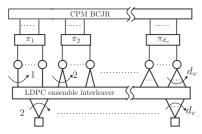
Fig. 2: LDPC code ensemble for joint detection and decoding.
