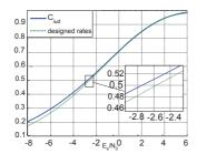
Fig. 4: Achievable and designed rates for GSM GMSK system.
