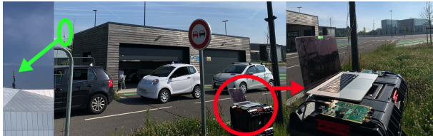
FIGURE 7. Experiment's equipments: In the green circle, the RSU installed in the campus and red circle the computer with the two USRP cards to simulate the attack messages.
