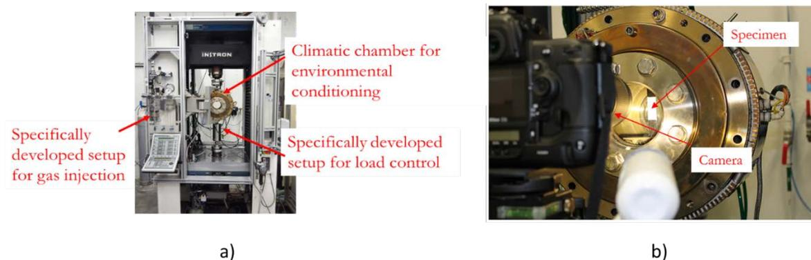
**Figure 2.** a) COMPTINN test setup developed @PPRIME b) detail of the climatic chamber.
