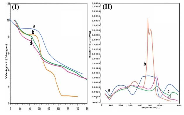
**Fig. 4** TGA & DSC curves overlay of samples. 3(I). TGA curves of (a) cefixime (b) QSM (c) unloaded microspheres of QSM/alginate (d) loaded microspheres of QSM/alginate containing cefixime. 3(II). DSC curves of (a) cefixime (b) QSM (c) unloaded microspheres of QSM/alginate containing cefixime.
