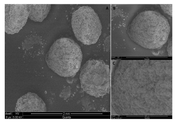
Fig. 5 Scanning electron microphotograph of microspheres of QSM-alginate containing cefixime (A) at 2.00 mm (B) 1.00 µm and (C) 400 µm.
