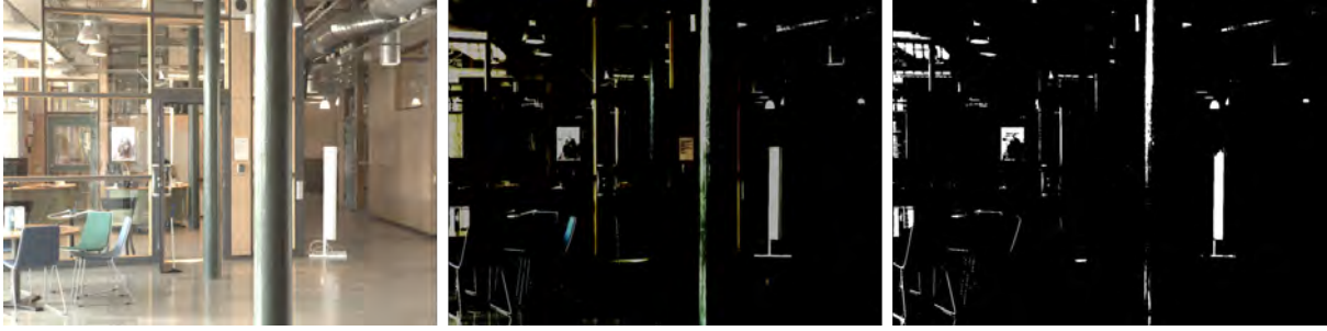
Figure 5: From Left to Right: Input Low Dynamic Range Image, Intensity Image on which the loss functions are computed, Image Mask after extracting the saturated regions of the image.
