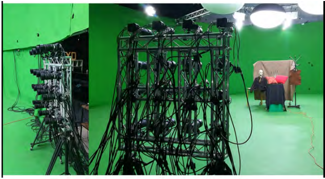
Figure 1: The ReVeRY camera built by our partner, XD Productions. It is a 16-image synchronised camera system. It is a wide-baseline camera array, with cameras apart of 20cm.
