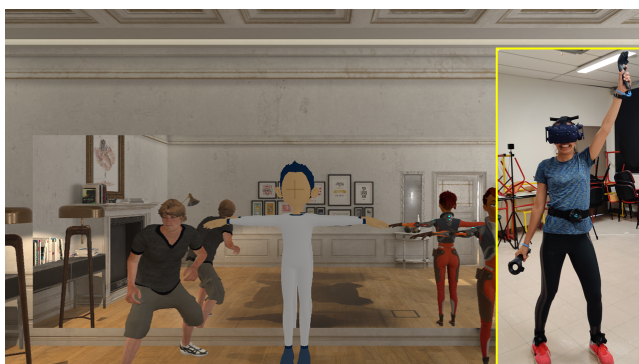
Figure 6: VR dance studio setup in Unity. [Inset] A participant wearing HTC Vive Wireless HMD with additional foot and hand trackers for full body tracking.
