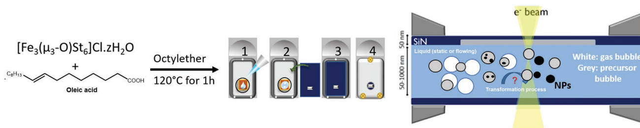
Figure 13. Left: schematic representation of the experimental protocol used for the preparation of LC-TEM experiments. First, 2.2 mmol in iron of iron stearate were mixed with 4.4 mmol of oleic acid in 20 mL octylether used as a solvent. The mixture was stirred and heated at 120 °C for 60 min without a reflux condenser in order to dissolve the reactants and remove the water residues. 1) One droplet of the previously heated solution was deposited over the bottom chip. 2 and 3) The top chip was placed rapidly over to avoid drying taking care of the proper alignment of the windows. 4) The lid was placed to close the system, fix both chips in position with the screws assuring the proper tightness to avoid any leaking to the TEM column. Right: scheme of the LC-TEM set-up and experiments. The thickness between the two SiN membranes is 150 nm.
