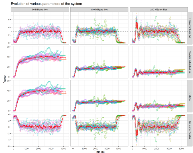
Fig. 3. Temporal evolution of the fileserver load (1 st row), the number of jobs submitted by CiGri (2 nd row), and the contribution of F (3 rd row) and the contribution of the error term (4 th row). Experiments run 10 times.
