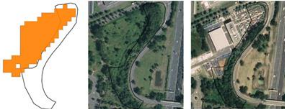
Figure 4: Example of errors referring to a change that only covers part of the initial polygon; LU polygons and associated data (at the left); aerial imagery in 2016 (in the middle); Pléiades imagery in 2019 (at the right); issued from Liu et al., 2020
