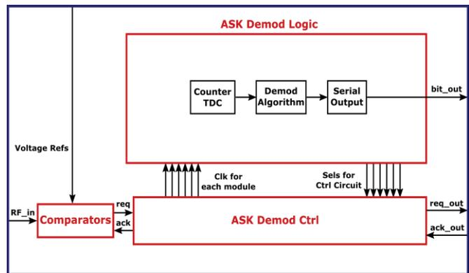
Figure 3: Schematic of the implemented testchip.
