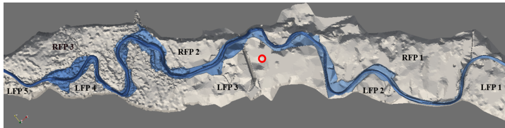
(c) 2D domain decomposition into river bed (blue) and surrounding floodplain divided in 8 sub-domains (grey shadowing) denoted by RFP and LFP (Right/Left FloodPlain) used for the lateral coupled model. A validation point is indicated with a red circle near Marmande and Coussin in LFP3 is the location.
