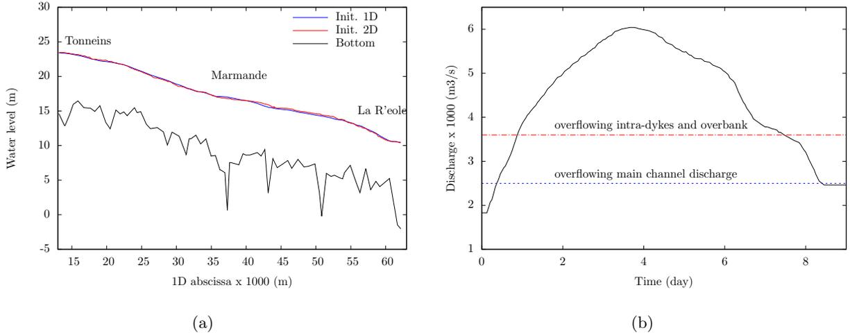
Figure 13: (a) Initial water level along the main channel resulting from permanent flow established with  $Q = 1830 \text{ m}^3/\text{s}$  in both 1D (blue line) and full 2D (red line) models. The 1D bathymetry is plotted with a black line. (b) Observed discharge at Tonneins; main channel overflowing is reached at  $Q = 2500 \text{ m}^3/\text{s}$ , overbank flow and intra-dykes overflow is reached at  $Q = 3600 \text{ m}^3/\text{s}$ .
