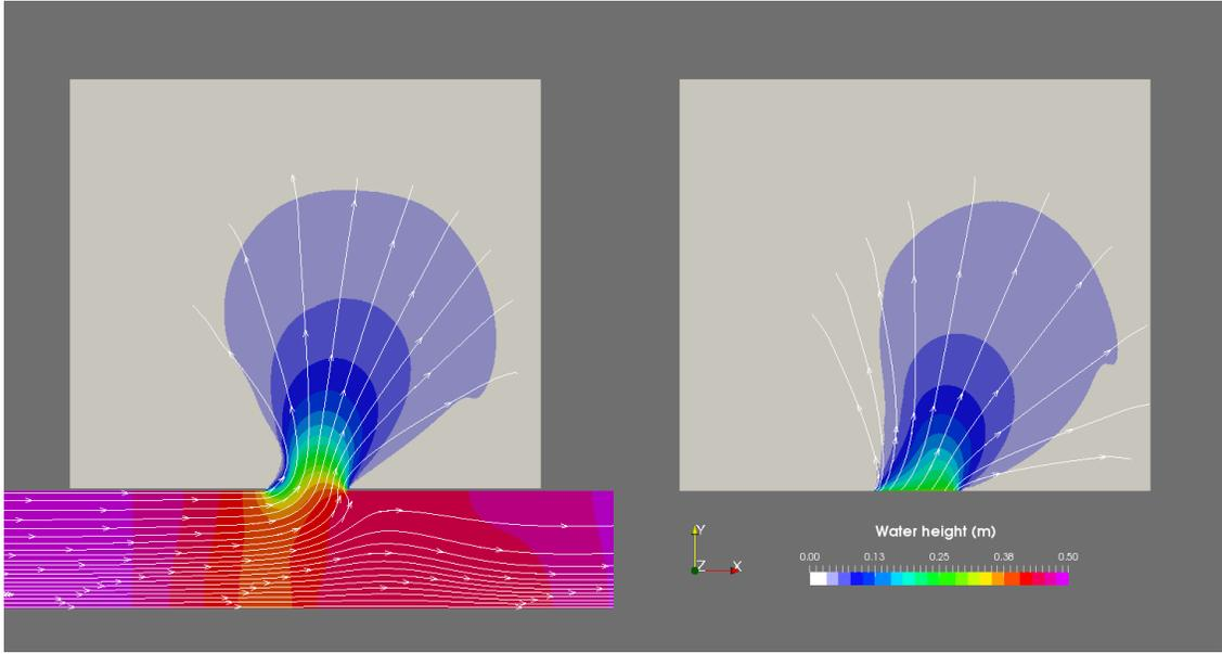
Figure 10: Water heights and stream traces for dyke-break test case at  $t = 1\text{s}$  given by the full 2D simulation (left plot, channel and floodplain) and the 1D-2D coupling (right plot, only floodplain). The bank model carried out about 10 sub-timeloops for each timestep  $\Delta t^{1D} = \Delta t^{2D} = 0.01\text{s}$ .
