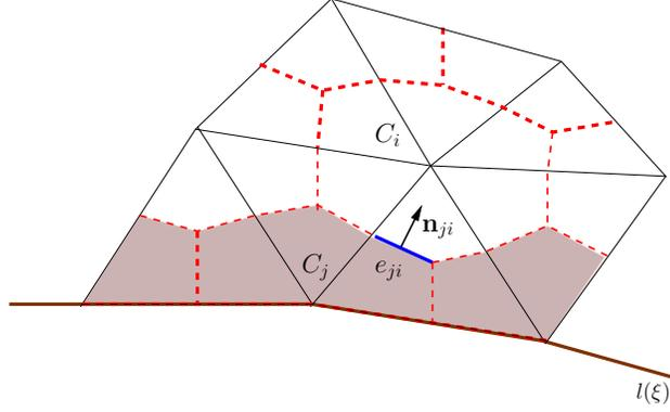
Figure 4: Zoom on the artificial boundary, i.e the boundary of buffer zone  $\Omega^b$  (shadow sub-domain) located inside the floodplain  $\Omega^{2D}$ . The red dashed lines stand for the dual mesh on which a vertex-centered finite volume discretization has been used.
