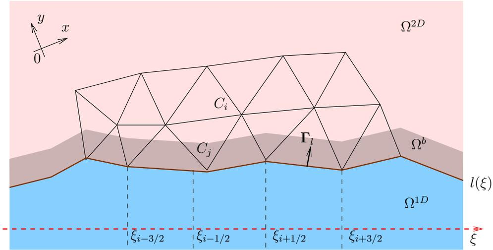
Figure 2: Sketch of river channel  $\Omega^{1D}$  and its left floodplain  $\Omega^{2D}$  discretized by 1D and 2D meshes respectively. The shadow sub-domain  $\Omega^b \subset \Omega^{2D}$  stands for the buffer zone along the lateral boundary  $l(\xi)$  that will be used for our coupling method.
