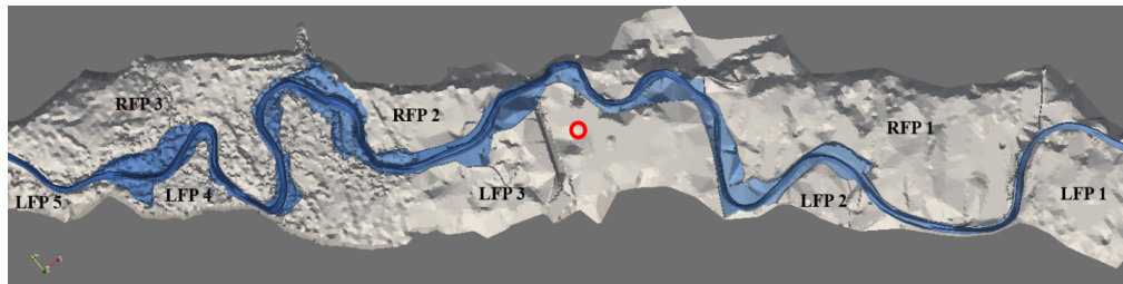
(c) 2D domain decomposition into river bed (blue) and surrounding floodplain divided in 8 sub-domains (grey shadowing) denoted by RFP and LFP (Right/Left FloodPlain) used for the lateral coupled model. A validation point is indicated with a red circle near Marmande and Coussin in LFP3 is the location.
