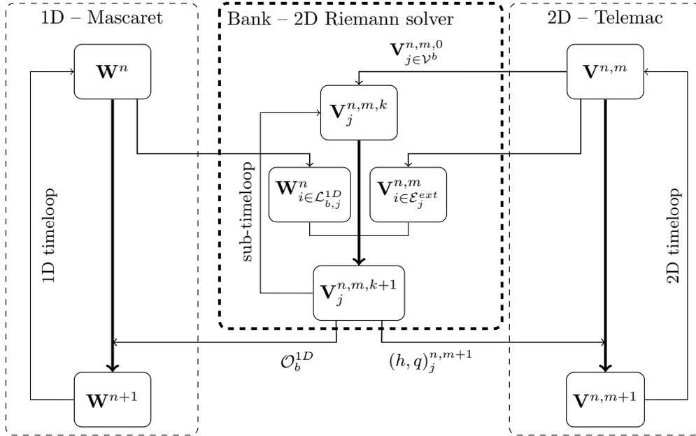
Figure 3: Schematic of the proposed lateral coupling procedure.
