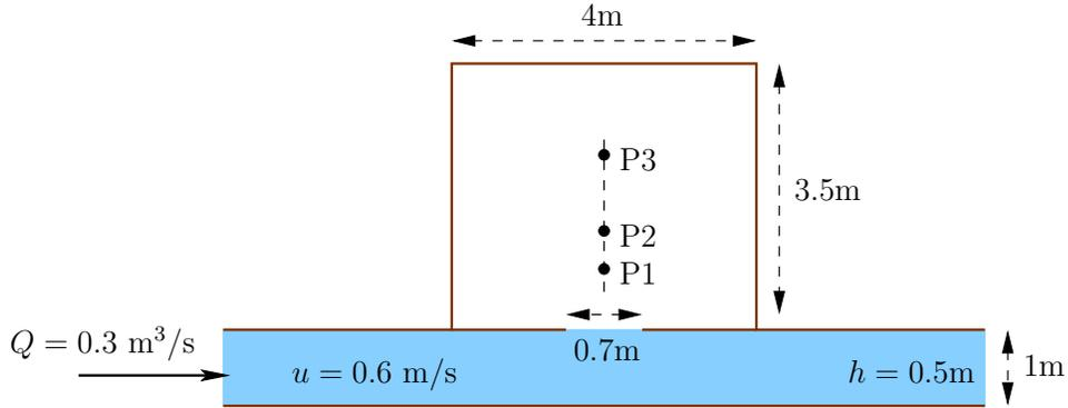
Figure 9: Physical model setup for dike-break test case: the length of dyke failure is 0.7m centered at  $(x = 0, y = 0)$ . Validation points in the flood plain are located at  $x = 0$  and  $y(P1) = 0.8$ ,  $y(P2) = 1.3$ ,  $y(P3) = 2.3$ .
