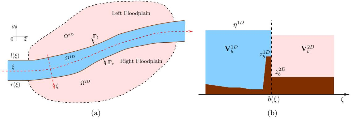
Figure 1: (a) Plan view for lateral coupling between the river and surrounding floodplains;  $(\xi, \zeta)$  represents the system of coordinates for the river. (b) Illustration of given data for the Riemann problem at the bank  $b(\xi)$ .
