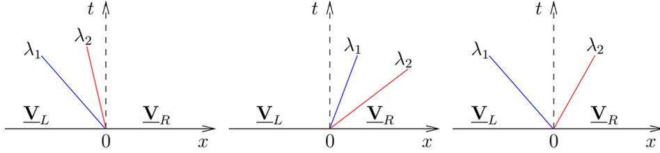
Figure 5: Riemann problems of the linearized shallow-water equations.
