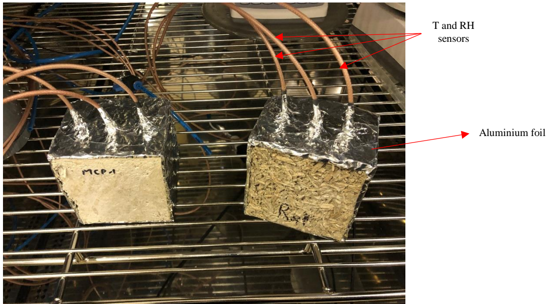
Figure 7. REF and PCM hemp concrete samples for the thermal performances test and the position of the RH and T sensors
