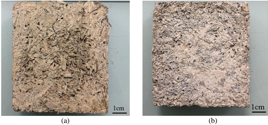
Figure 4. (a) REF and (b) PCM hemp concrete samples for the thermal conductivity measurement
