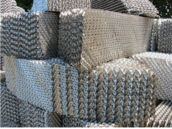
FIGURE 4. PHOTOGRAPH OF STRUCTURED PACKINGS (WIKIMEDIA COMMONS, AUTHOR: LUIGI CHIESA).
