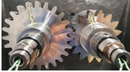
Figure 6. Thermocouple sensors stuck on gears tooth
