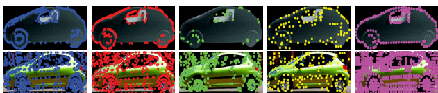
Fig. 5: Features extracted in the depth (row 1) and the real image (2) with: MCS (column 1), PCI proposed in [8] (2), SIFT (3), Harris (4) and Edge detector proposed in [12] (5).
