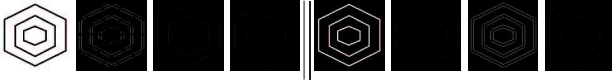
Fig. 2: Curviness saliency of two shapes (columns 1, 5) with minimum (2, 6), maximum (3, 7) and the difference between maximum and minimum eigenvalues (4, 8).
