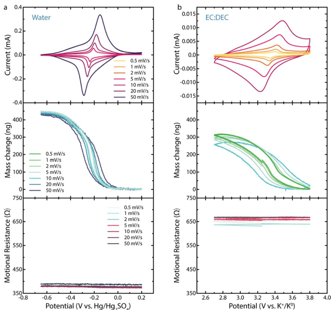
**Figure 2.** Cyclic voltammetry of a 100 nm thick PB film at different scan rates, in (a) 0.25 mol.L<sup>-1</sup> K<sub>2</sub>SO<sub>4</sub> in H<sub>2</sub>O (pH 3.5) and (b) 0.5 mol.L<sup>-1</sup> KPF<sub>6</sub> in EC:DEC. Current (top), mass changes (middle) and absolute motional resistance (bottom) were simultaneously measured. The frequency change was converted into mass change, using Sauerbrey equation. The fifth cycle is here represented for each scan rate.
