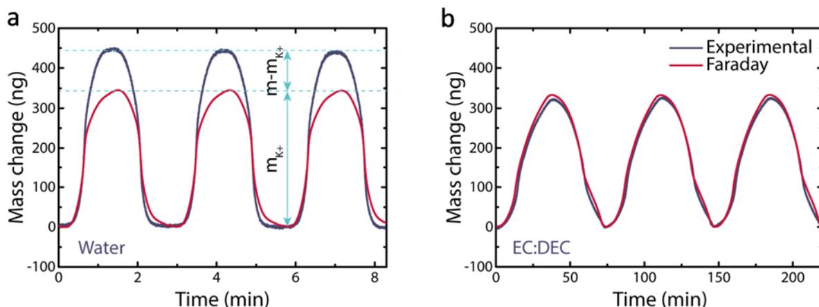
**Figure 5.** Experimental (EQCM) and electrochemical mass (Faraday) comparison calculated for a 100 nm thick film (a) in 0.25 mol.L<sup>-1</sup> K<sub>2</sub>SO<sub>4</sub> (pH 3.5) water-based electrolyte during a CV at 10 mV.s<sup>-1</sup> and (b) in 0.5 mol.L<sup>-1</sup> KPF<sub>6</sub> EC:DEC-based electrolyte during a CV at 0.5 mV.s<sup>-1</sup>. The corresponding EQCM data are presented in Figure 2.
