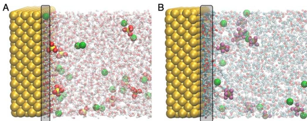
**Figure S8.** Representative snapshots extracted from the MD simulations of K<sub>2</sub>SO<sub>4</sub> in H<sub>2</sub>O (A) and KPF<sub>6</sub> in EC/DEC (B). Au atoms are represented in dark yellow, K<sup>+</sup> cations in green, and SO<sub>4</sub><sup>2-</sup> and PF<sub>6</sub><sup>-</sup> anions in yellow/red and brown/violet, respectively. Solvent molecules belonging to the first layer in contact with the Au surface are highlighted.
