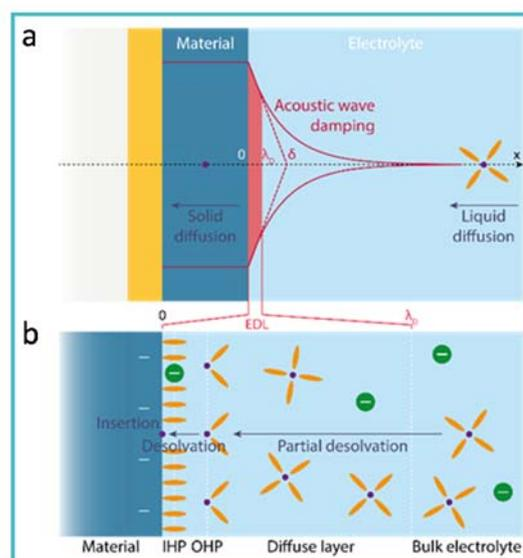
**Figure 3.** Schematic representation of the insertion of an alkali metal cation in a host material. (a) Comparison between the penetration depth of acoustic wave from the QCM to the solution ( $\delta$ ) and the electrochemical double layer characteristic length ( $\lambda_D$ ). (b) Close-up snapshot of the electrochemical double layer during cation insertion.
