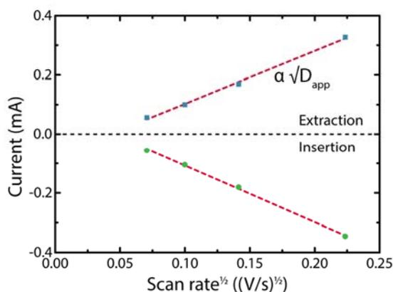
**Figure S3.** Apparent diffusion coefficient determination of  $K^+$  during insertion and extraction in a Prussian Blue film (100 nm) in  $K_2SO_4$  0.25 mol.L<sup>-1</sup> aqueous electrolyte by the Randles-Sevcik equation.
