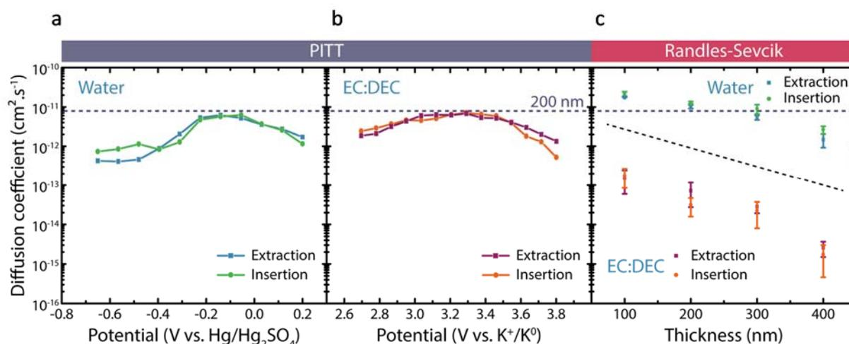
**Figure 4.** Comparison of the solid diffusion coefficient of potassium ion in PB films of 200 nm, obtained (a, b) by PITT and (c) by the Randles-Sevcik equation. For the PITT results obtained at different film thicknesses refer to Figure S2.
