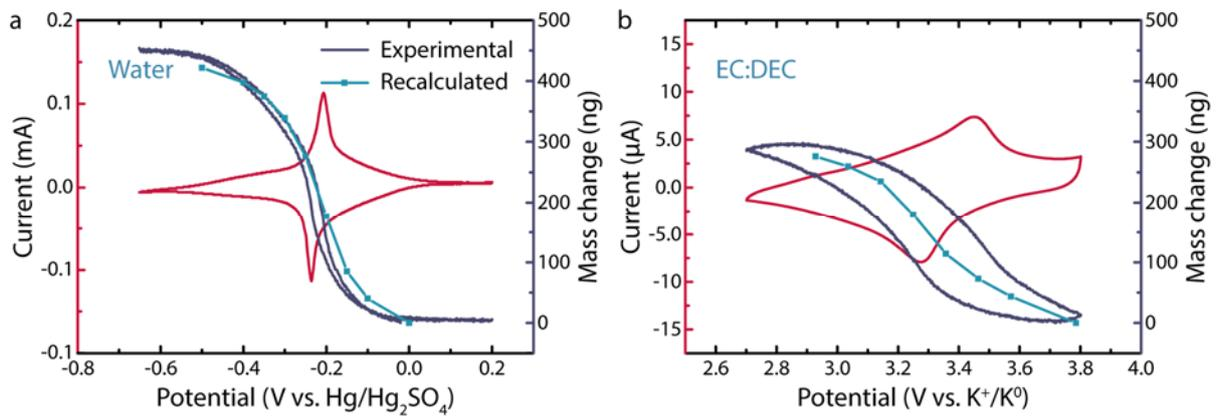
**Figure S7.** Comparison of the mass variation by classical EQCM measurement at  $5 \text{ mV.s}^{-1}$  with recalculated mass variation by *ac*-electrogravimetry in (a) water and (b) ED:DEC-based electrolytes.
