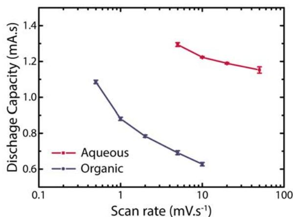
Figure S5. Rate capability assessment of the 100 nm thick PB film in aqueous (0.25 mol.L<sup>-1</sup> K<sub>2</sub>SO<sub>4</sub> in H<sub>2</sub>O (pH 3.5)) and non-aqueous electrolyte (0.5 mol.L<sup>-1</sup> KPF<sub>6</sub> in EC:DEC) by means of the discharge capacity.
