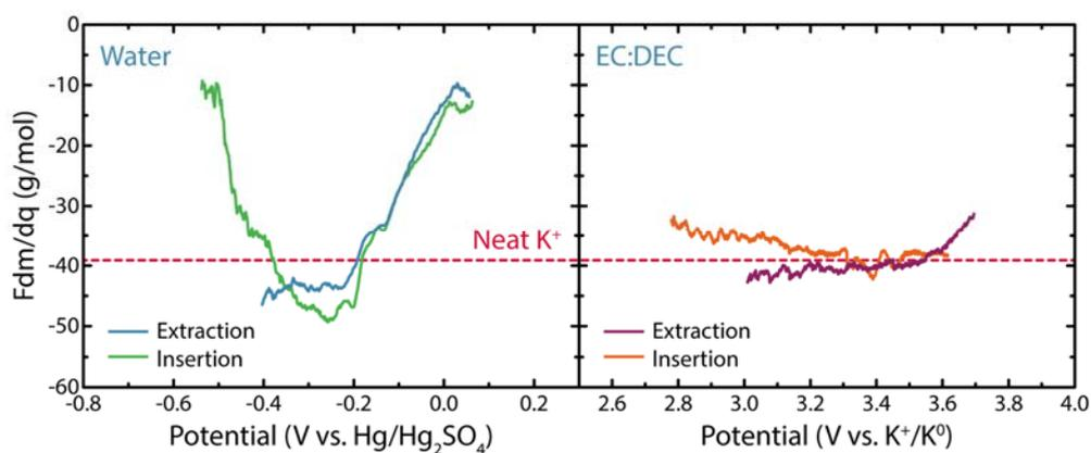
Figure S6.  $F\Delta m/\Delta Q$  calculated for a 100 nm thick film (a) in 0.25 mol.L<sup>-1</sup> K<sub>2</sub>SO<sub>4</sub> (pH 3.5) water-based electrolyte during a CV at 10 mV.s<sup>-1</sup> and (b) in 0.5 mol.L<sup>-1</sup> KPF<sub>6</sub> EC:DEC-based electrolyte during a CV at 0.5 mV.s<sup>-1</sup>. The corresponding EQCM data are presented in Figure 2.
