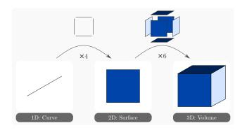
Fig. 4: Illustration of the essential geometric operations resulting in a volumetric cube.
