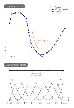
Fig. 2: Physical and parametric spaces for a quadratic B-Spline curve in  $\mathbb{R}^2$ . The associated knot vector is defined as  $U = \{0, 0, 0, 1/7, 2/7, 3/7, 4/7, 5/7, 6/7, 1, 1, 1\}$ .
