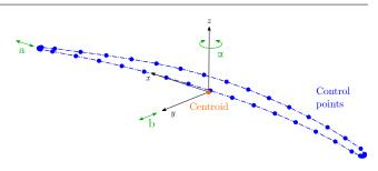
**Fig. 11:** Illustration of the authorised motions for one section for the stacking axis shape parametrisation. Only the exterior control points of the section are represented for clarity.
