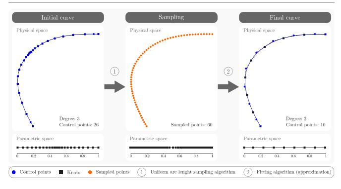
Fig. 7: Curves re-parametrisation steps. The process is illustrated for a leading edge curve; here the interest of obtaining a coarser parametrisation appears clearly.
