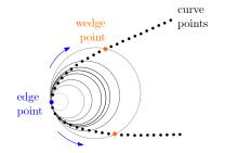
**Fig. 6:** Schematic view of the process of fitting the edge points to a sphere. The operation is illustrated in the 2D case for clarity.
