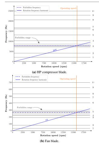
**Fig. 10:** Initial Campbell diagrams of the HP compressor (a) and fan (b) blades. The dashed line represents the frequency value we seek to avoid. This value corresponds to a given harmonic of the rotation speed we consider (vertical orange line on the figures). The shaded area corresponds to a 15% margin around this value. The indices on the right-hand part of the diagrams correspond to the vibration modes indices.
