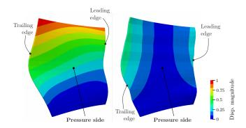
Fig. 13: Displacement fields for the initial (left) and optimised (right) geometries after compliance optimisation on the HP compressor blade.
