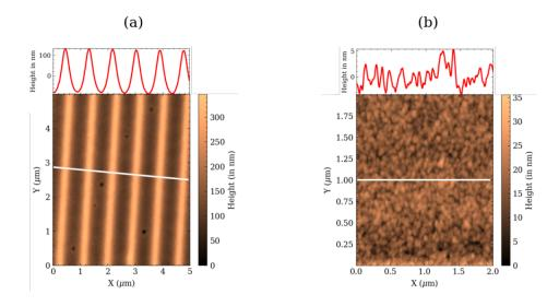
Figure 6. AFM images of (a): profile of the line for the deep gold grating ( $\Lambda=890$  nm, d=215 nm); (b) profile of the flat gold coated surface.
