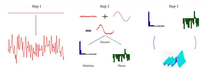
Figure 1. Scheme of the three different modeling steps for the computation of the theoretical response of rough gratings.
