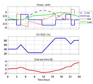
Fig. 7. Simulation results for bidirectional smart charging scenario.
