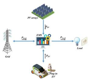
Fig. 1. Typical configuration of a PV-assisted PEV charging station.
