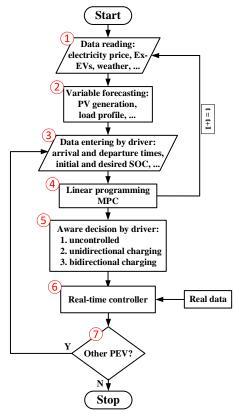
Fig. 2. Flowchart of the proposed smart charging algorithm.
