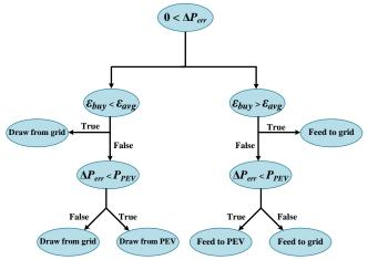
Fig. 3. Rule-based real-time control scheme [5].
