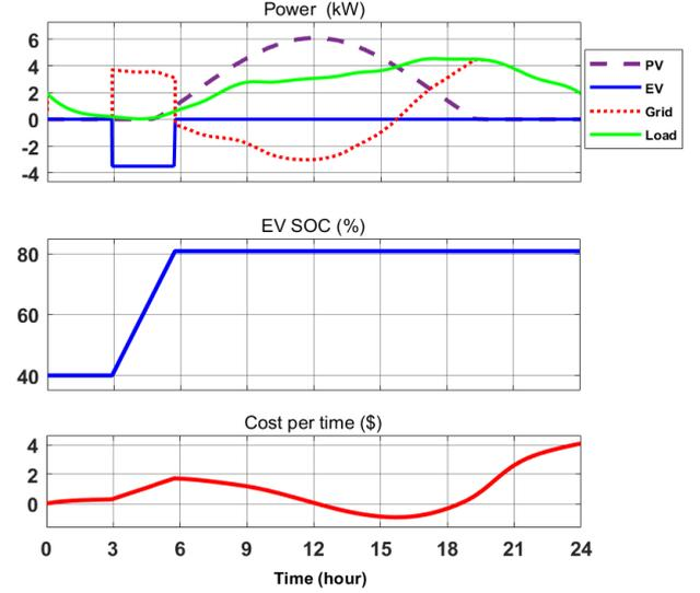
Fig. 5. Simulation results for uncontrolled charging scenario.
