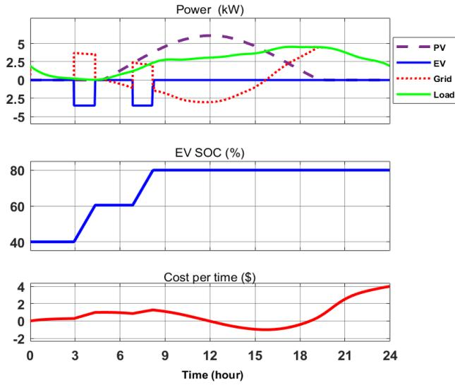
Fig. 6. Simulation results for unidirectional smart charging scenario.
