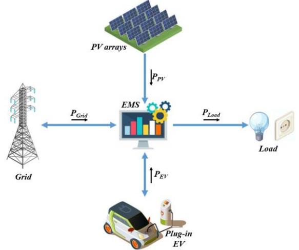
Fig. 1. Typical configuration of a PV-assisted PEV charging station.
