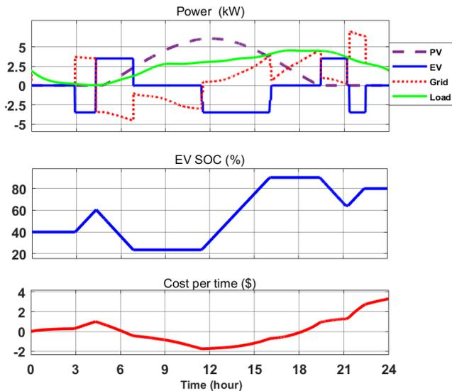
Fig. 7. Simulation results for bidirectional smart charging scenario.
