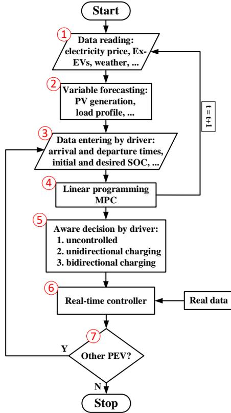
Fig. 2. Flowchart of the proposed smart charging algorithm.
