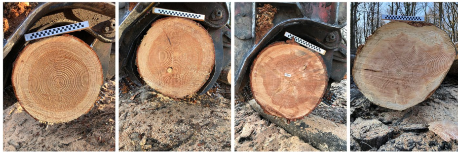
Fig. 4 Large ends of logs A12d, B05c, C04b, and D04a (from left to right) at the logyard. The image of log D04a was taken directly on the long log; the others were taken with the log held by the harvester. The 25-cm-long scale was used to calibrate each image
