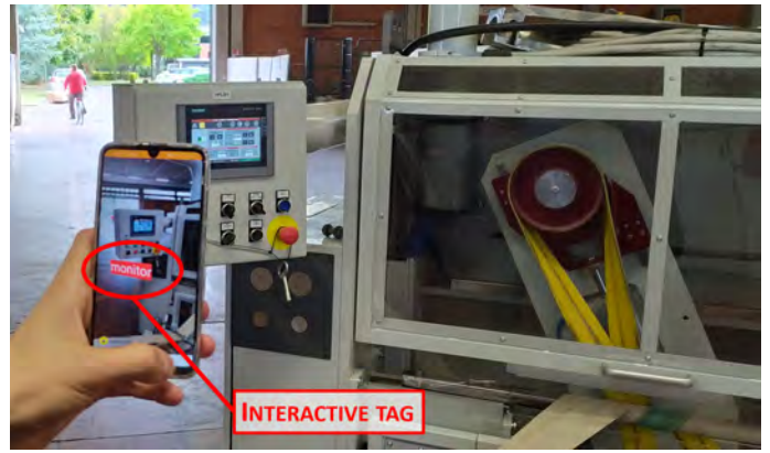
Fig. 2. An AR interactive tag relative to a complex component of the tissue converting line.
