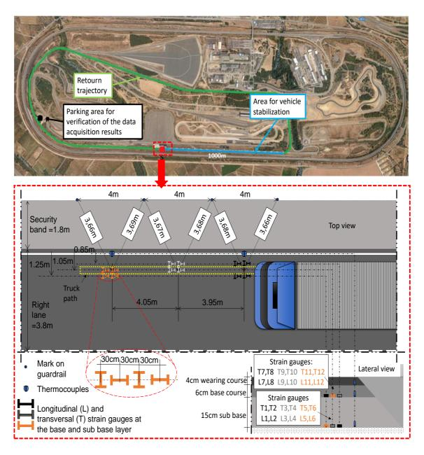
Fig. 1. IDIADA test track and instrumented test section.
