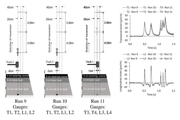
Fig. 11. Analysis 2: Reproducibility, considered truck speed = 60 km/h, winter campaign, Individual Configuration, Transversal (T) and Longitudinal (L) strain gauges.
