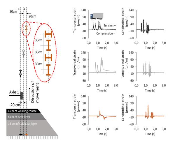
Fig. 7. Horizontal strains obtained from run 8 for Truck 1 under individual configuration (Summer campaign, Truck speed = 60km/h, Strain Gauges Depth = 25 cm, Y1 = 0.65m, truck distance from the central strain gauges set = -20cm).
