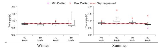
Fig. 16. Inter-truck time gaps in the platoon configuration.
