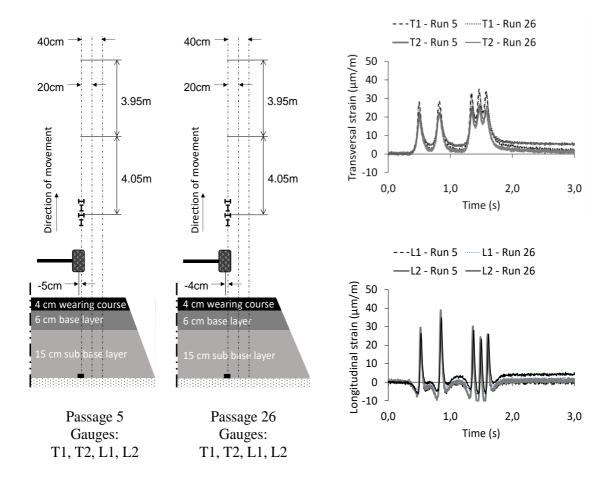
Fig. 10. Analysis 1: Repeatability, Truck 1, Truck speed = 60 km/h, Individual Configuration, Transversal (T) and Longitudinal (L) strain gauges, winter campaign.
