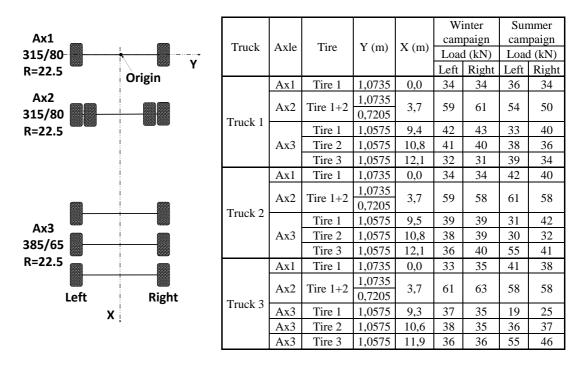
Fig. 4. Axle geometrical configuration and weight for each truck.
