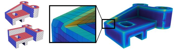
Figure 12: In some cases, Evocube finds a low-distortion labeling that assigns the same label across a feature edge. In our current postprocessing pipeline and similarly to other polycube-based methods, such feature edges are not always preserved.
