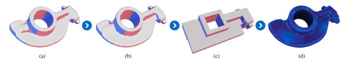
Figure 4: Starting from a triangular mesh representation of a 3D shape, (a) we generate an initial non-optimal and potentially invalid labeling using a graph-cut method [LVS\*13]; (b) this labeling is then refined to be valid within our Evocube framework; (c) we generate a polycube with topology matching our labeling, and (d) a grid-like mesh is extracted, padded and morphed back onto the initial 3D shape.
