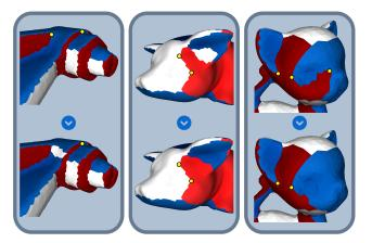
Figure 7: Base mutations in our genetic framework. Turning points are highlighted in yellow. From left to right: directional path, chart removal, and chart propagation.
