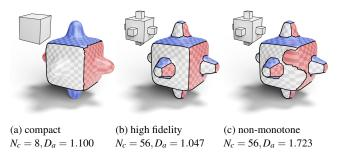
Figure 3: Illustration of labeling properties and associated polycubes. We report the number of corners in the polycube  $N_c$  and the area distortion  $D_a$  [THCM04].
